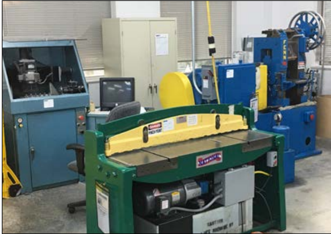
Figure 2. One of Secat’s labs showing a CNC machine, shear, and rolling mill.
